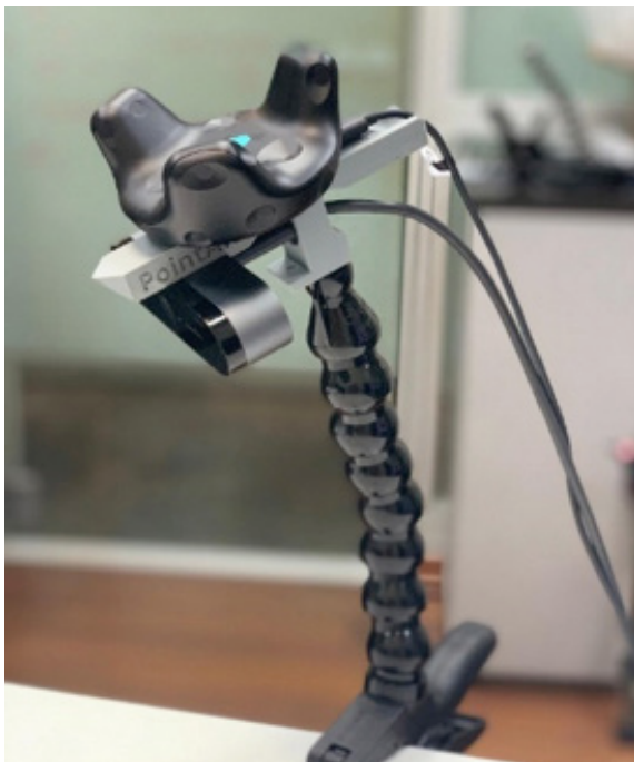
Figure 4. A PointAR unit equipped with IR-based sensors for tracking and a standard Logitech 4k web camera. PointAR is available in several versions to support different use cases, ranges and accuracy demands.
