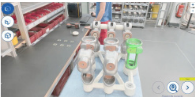
Figure 7. An AR-enhanced work instruction solution for an assembly station at the Siemens Gas and Power factory, gas-insulated switchgear manufacturing line in Berlin, Germany.
